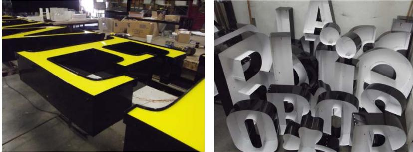
A channel letter is a 3-D component in signage. Typically these are used on the store front. A “can” is made in the shape of your logo or lettering with aluminum, acrylic and internal illumination. The back side of the can is cut using the design created by our art staff and then sent to a computerized router table. This gives a precise shape for the finished “Channel”.
